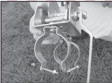
1. Assemble winch by placing handle on - tighten. Attach clamps to back of winch with machine screws and nuts.
