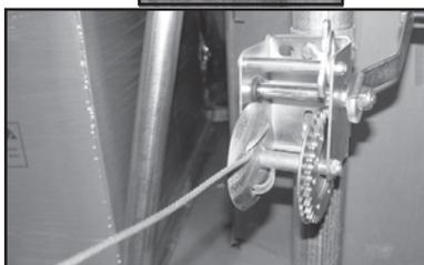
4. Unwind the cable from the winch spindle. Take note of how the cable is secured to the winch. Before removing the cable from the side wall of winch, mark the cable (use a black marker or tape) at the point where the cable first enters the side wall (Approximately 13 inches of cable is required to wrap around the sidewall of the winch to secure the cable).
