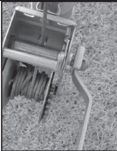
2. Place the winch on the pole at the location you want to operate it. Make sure the winch is placed on the pole with the top facing the sky. As shown in photo. We recommend the winch be placed somewhere between two (2) to four (4) feet above the ground.
