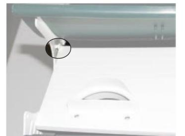
**Step 19:** The four door panels are attached by inserting the end tabs through the molded holes in the side panel as shown. The door panels will swing up. Press the floor tabs behind each door panel until they snap into place.
