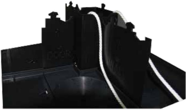
**Step 11:** Place the second floor a top the dividers. Be sure the floors are turned in the same direction. Push the tabs of the standing dividers into the corresponding holes. Insert the second Pillar (around ropes as in step 1) add dividers on the second floor exactly as the first floor (Steps 6-10).
